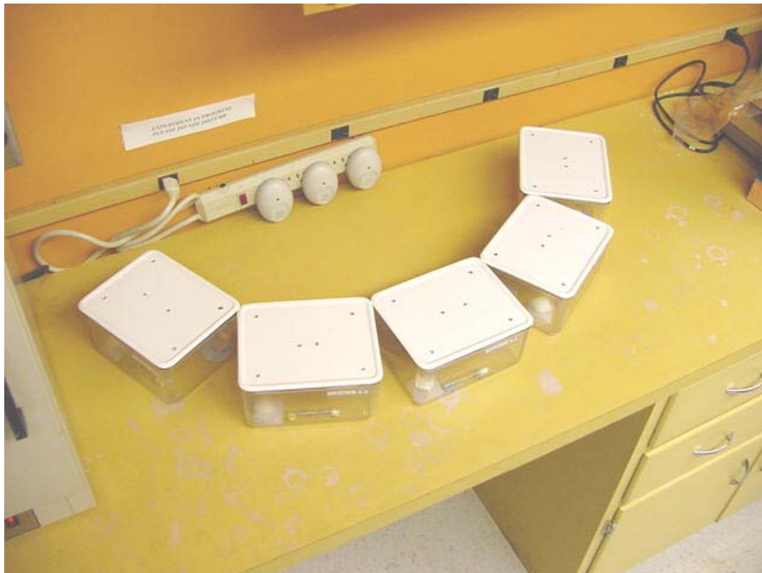
Figure 3-6. Five colony boxes placed near three electronic pest repellers
